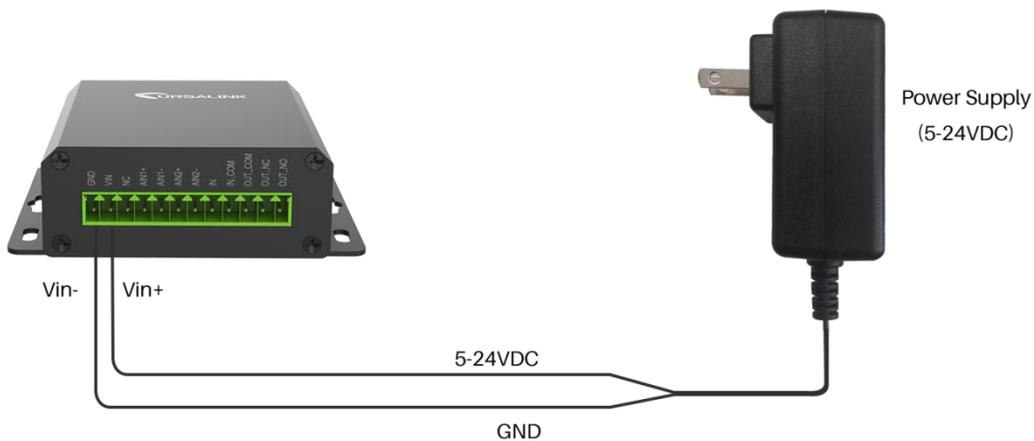
For industrial applications, it is advised that the Ursalink UC1122 should be installed into its own metal housing and be powered from a separate power supply (as opposed to sharing one with other equipment).
